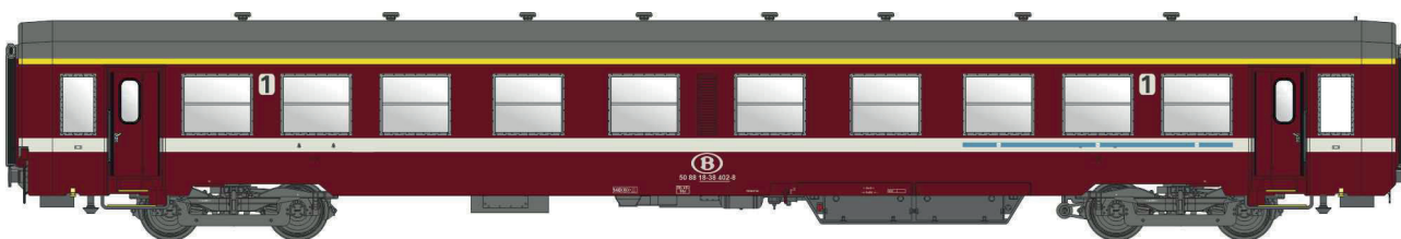
MW40039 A, bogies Y24
